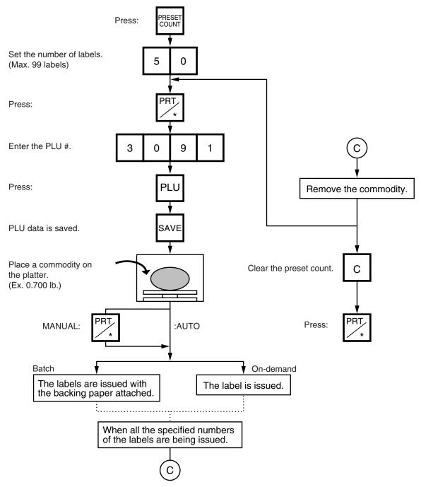
**NOTES:** 1. A batch issue means to print labels continuously with the backing paper attached. On-demand issue means to print label one by one.
